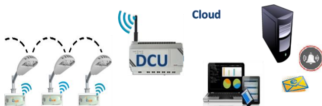
Wireless street light connected to cloud and mobile through DCU
