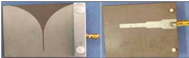
The fabricated antenna for Through wall imaging radar
