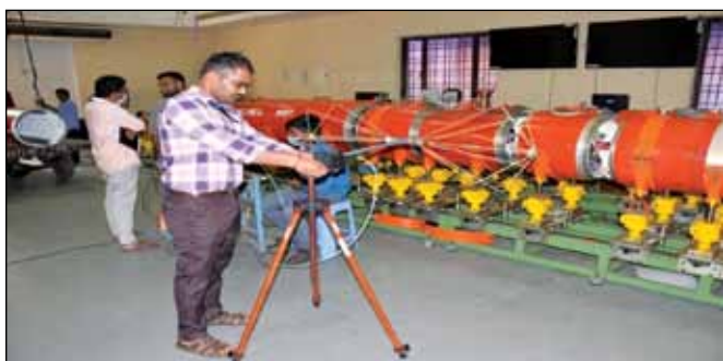
EMI/EMC testing of Electrical Heavy Weight Torpedo (EHWT)
