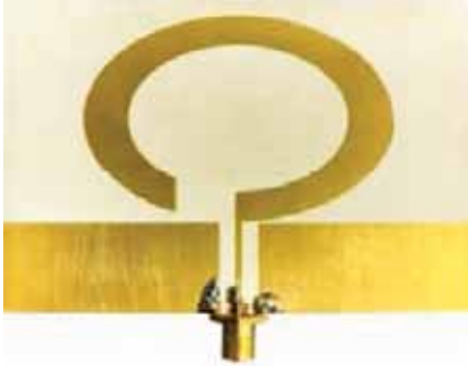
Tri-band NavIC antenna (L1, L5 &S)
