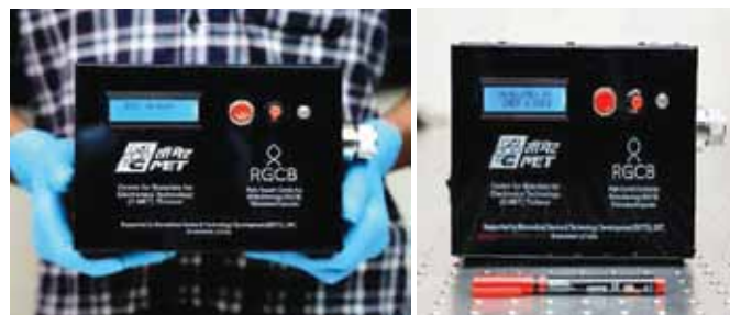
Plasmonic based portable Biosensor with disposable chip
