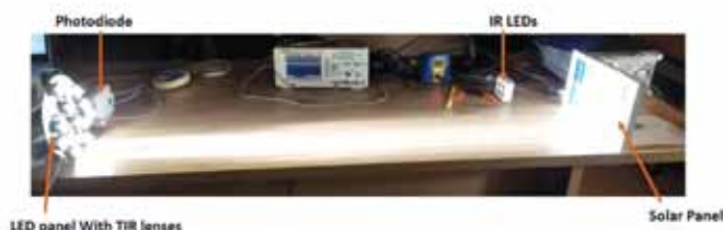
Fig. LiFi Outdoor Deployment Architecture (lab setup)
