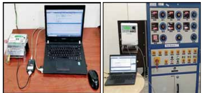
Smart Energy Meter for testing of DLMS/COSEM software testing
