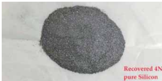
Recovered 4N pure Si from end-of-life Si solar cell
