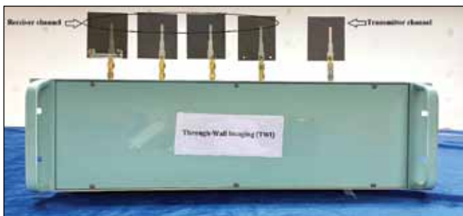
Antennas mounted on top of the TWI unit
