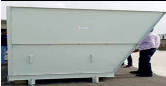
Sodar system installed at SAMEER Mumbai terrace
