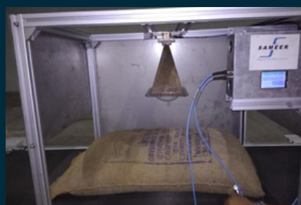
MOISTURE MEASUREMENT CONVEYER
