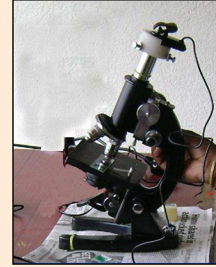
Microscope with camera interface
