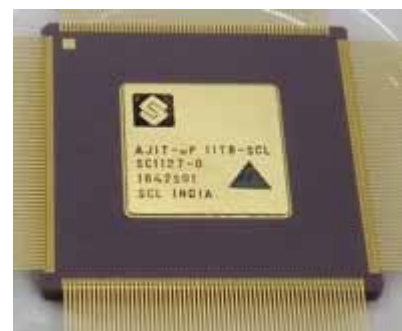
32-bit Microprocessor by IIT Bombay fabricated at SCL, Mohali Foundry
