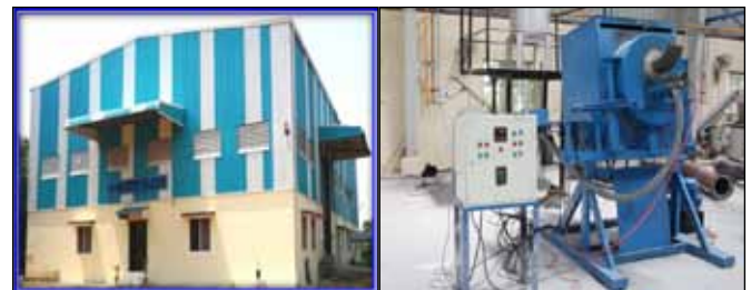
Shed and Front Fired Rotary Tilting Furnace (FFRTF) at e-waste facility
