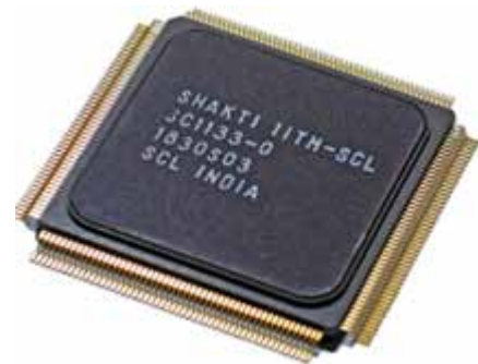
64-bit Microprocessor by IIT Madras fabricated at SCL Mohali Foundry
