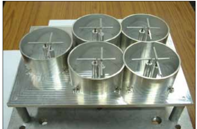
Fabricated S-band Reconfigurable Telemetry Antenna.
