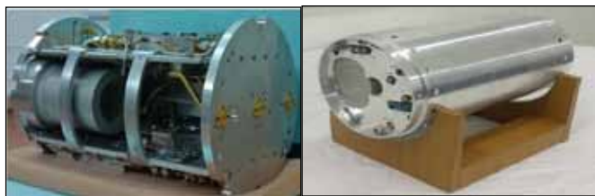
Perspective view of the developed W-band transceiver
