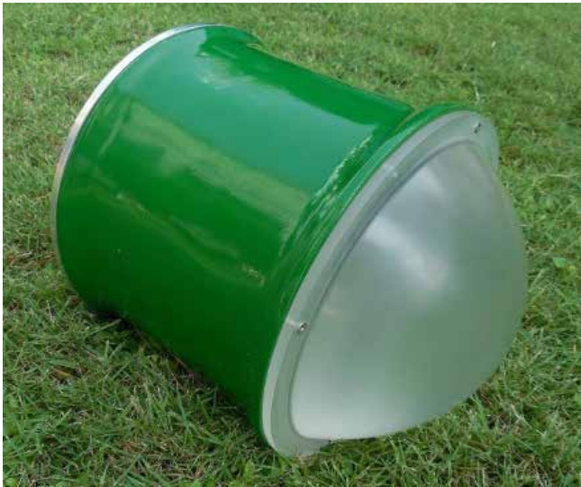
Fig: Indigenously developed Lens antenna with elliptic profile at 280 Ghz for 6G THz test bed
