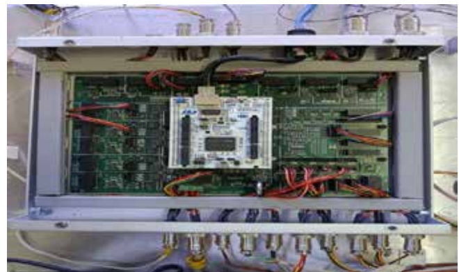
Fig: Data Acquisition system and Control unit for Dual band Radiometer
