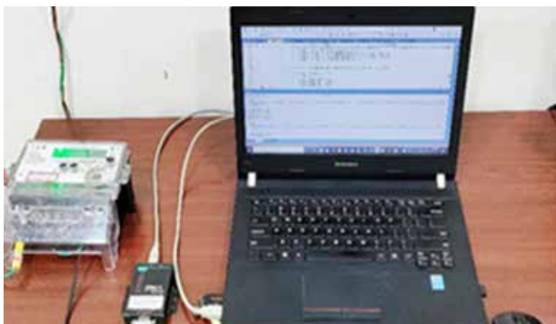
SMITHA: Software tool for testing and verifying smart-meter communication protocols
