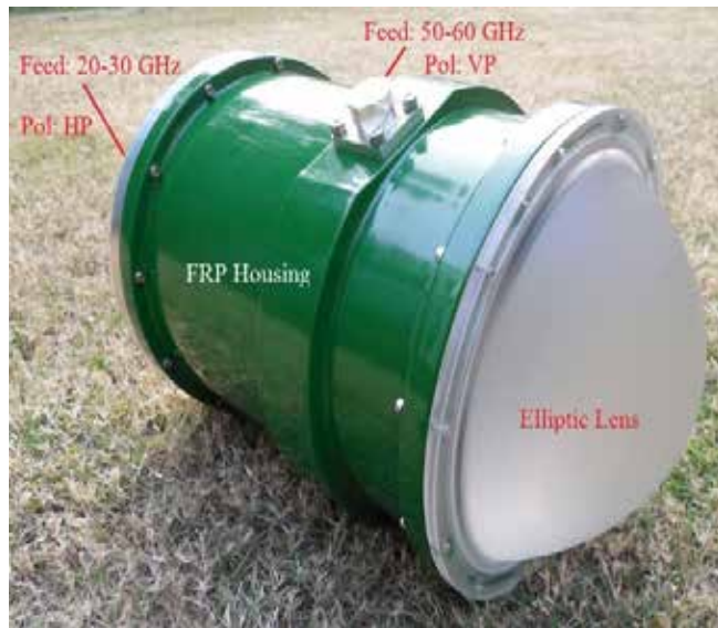
Fig: The dual-band lens antenna for radiometer application
