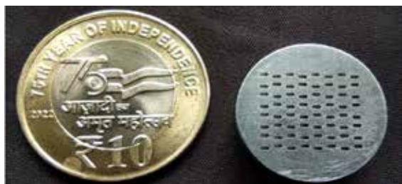
Fig: Slotted array antenna developed at 140 GHz for 6G Sub-THz Wireless communication with Intelligent Reflecting Surfaces (IRS).
