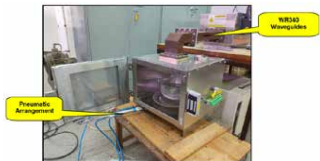
Fig: 1 kW microwave oven for radioactive gel drying.
