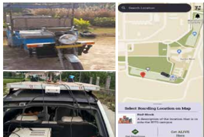
Autonomous Last Mile Vehicle (ALIVE) with GUI Based interface with Android App
