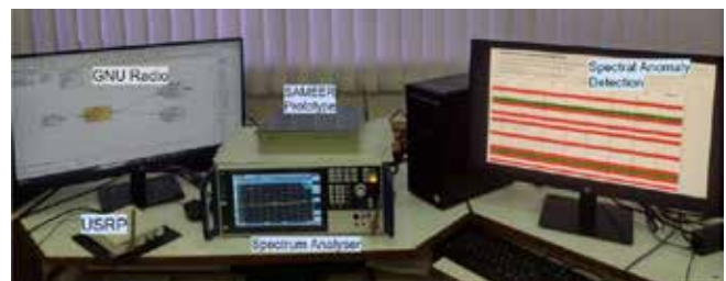
Fig: Lab validation setup for spectral anomaly AI model detection using SAMEER prototype.
