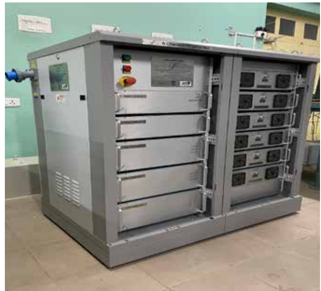
Fig: 6 channel 100W source for Microwave hyperthermia treatment installed at IIT Madras
