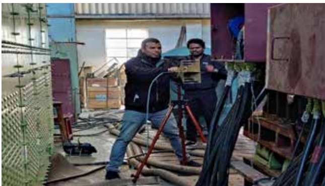
Fig: EMI/EMC Qualification of 1 MW Rotary Main Motor Generator (RMMG)
