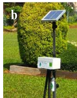
(a) Soil moisture sensors; (b) Soil moisture sensing device
