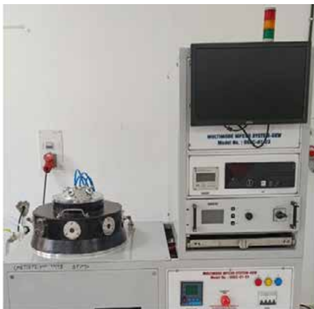
Microwave Plasma Chemical Vapor Deposition system for Quantum Grade Diamond Substrates
