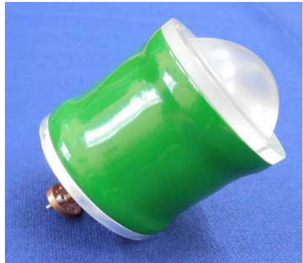
Fig: Lens antenna at 140 GHz for 6G Sub-THz Wireless communication with Intelligent Reflecting Surfaces (IRS)
